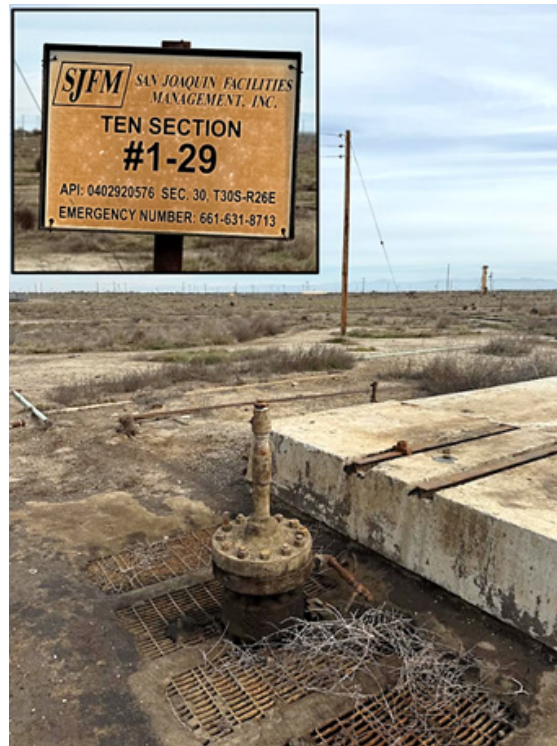
The discovery well at the Ten Section oil field, 1-29. This well had an initial production of 744 barrels of oil per day and 12.45 million cubic feet of gas per day. These rates would be repeated across the field during its development phase through WWII and experienced at surrounding follow-on discoveries as well.
