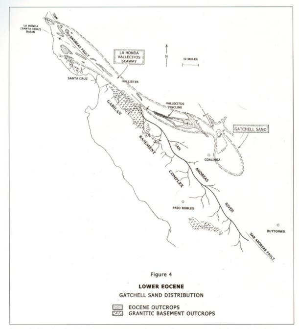
**Figure 4.** Map showing the Gabilan granitic sand source, the proposed southerly flowing Early Eocene La Honda-Vallecitos seaway, and the subsurface depositional limits of Gatchell-Lower McAdams sands in the San Joaquin basin.
