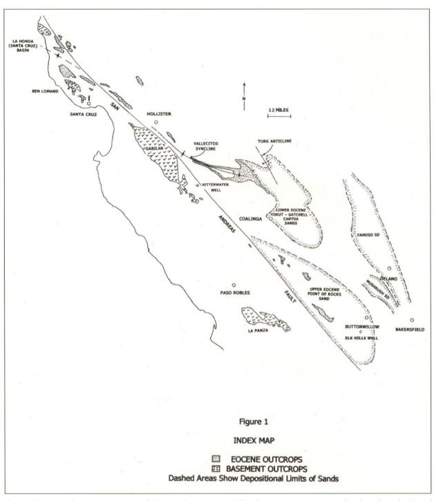
**Figure 1.** Map showing Lower and Upper Eocene sand distribution, outcrops, and subsurface limits of deposition. In the La Honda basin a full and uninterrupted sequence of Eocene is present.
