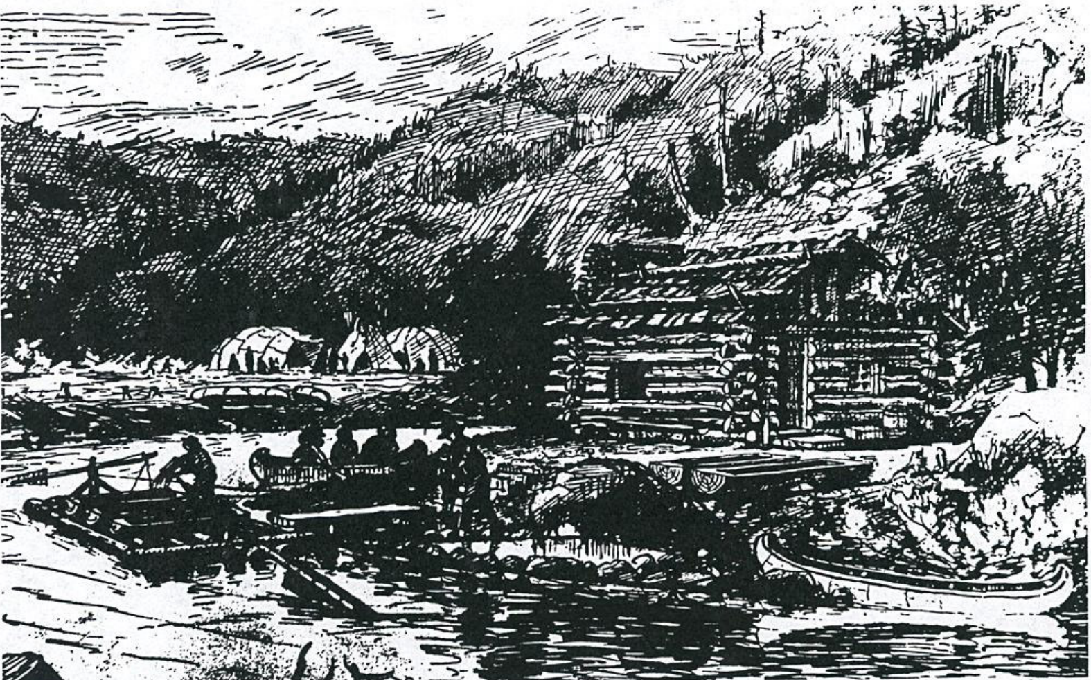
COLLECTING OIL ON OIL CREEK, 1810. In 1810 J. Francis Waldo made a sketch of some men skimming petroleum from an spring on Oil Creek near the present site of Titusville. The oil is being placed in hollowed-out-logs on a raft to be floated down the Creek and the Allegheny River to Pittsburgh.
